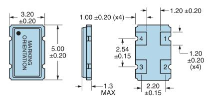
Note: Pin 1 Chamfer not shown.
